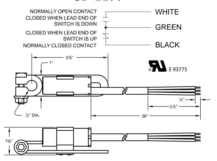
RATINGS: 2 AMPS @ 120 VAC 1 AMP @ 240 VAC STORAGE: NORMAL SHEL TYPE STORAGE, TEMPERATURE BETWEEN -38°F & 105°F OPERATING ANGLE:
