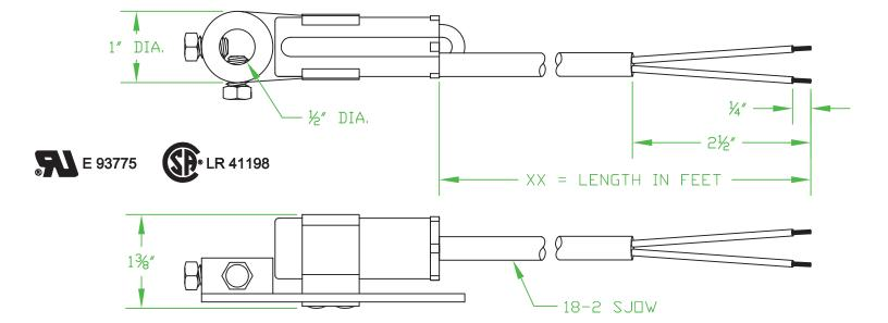
RATINGS: 1 AMP @ 120 VAC 1 AMP @ 24 VDC STOREAGE & OPERATION: NORMAL SHELF TYPE STORAGE, TEMPERATURE BETWEEN -38°C AND 90°C
